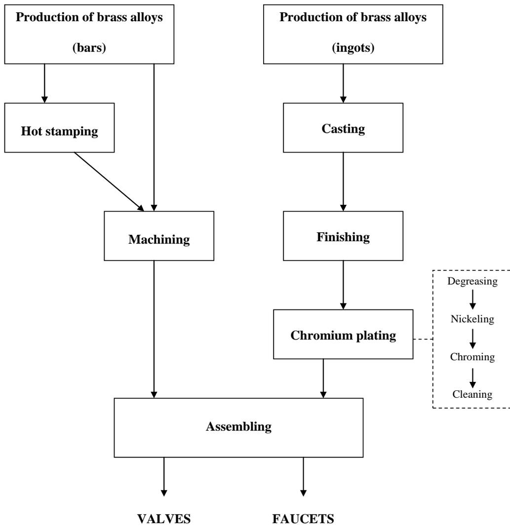
*Fig.1. Example of structured technology model of production of valves and faucets*
