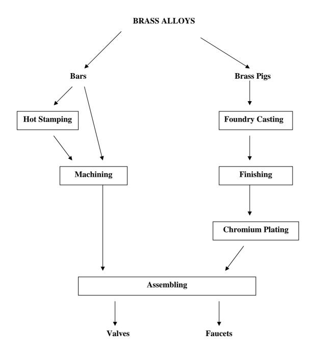
Fig. 1. Technological operations in production of faucets and valves
